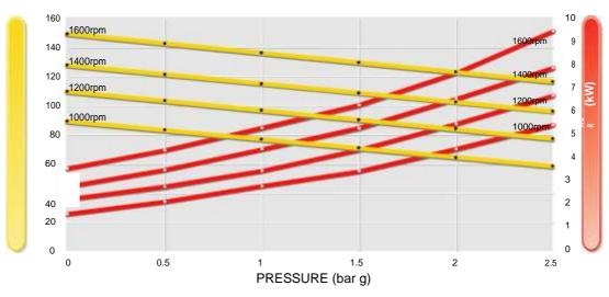
Flow measured in accordance with BS1042/ISO 5167-1/BS ISO TR 15377 and referred to standard ambient conditions (1013 mbar, 20°C)
